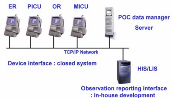
Figure 1. A diagram of networked POC arterial blood gas analyzer and connecting system
